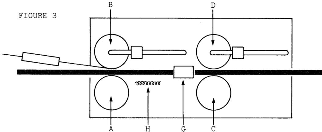
The guides and rollers soon reach a high equilibrium temperature whilst the first running adjustments are being made and, as a consequence there is no need to make special provision for heating them. In practice they receive a considerable amount of stray radiation from the infrared heater.
