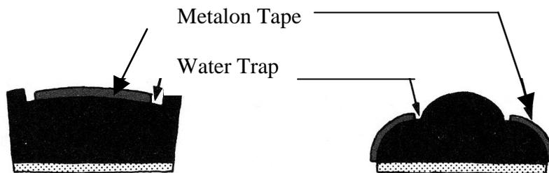
The diagram below shows extrusions where the edges of the tape are protected against damage by being buried in the extrusion itself or by being wrapped underneath and covered by the double-sided adhesive mounting tape.
